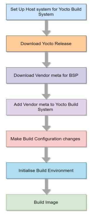
Figure 2: Workflow: Building Linux Image using Yocto
